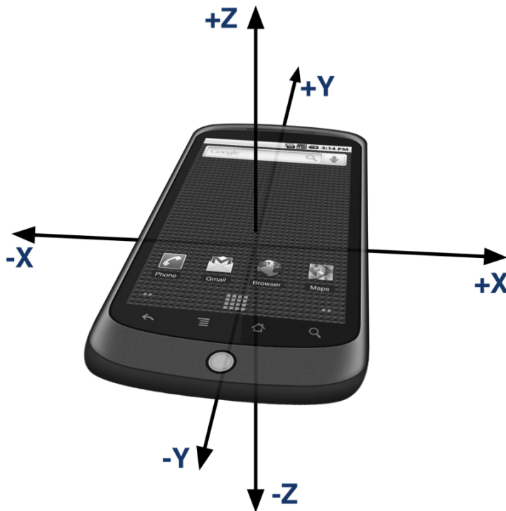
Figure 7–8. The accelerometer axes of an Android phone
